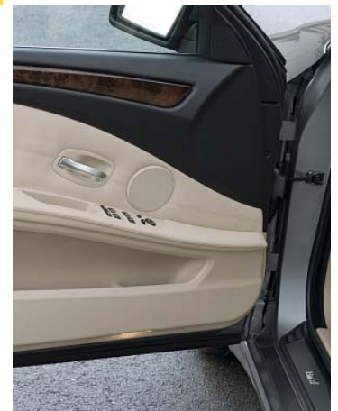
By introducing machinery and process innovations, Johnson Controls managed for the first time ever to apply a two-color foil to a single-component substrate made of natural fibers.
