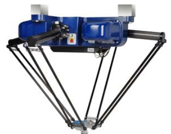
The Adept Quattro robot, equipped with four arms, can handle up to 240 parts/minute and attain accelerations of 200 meters/square second for loads up to 2 kilograms. Image: © F. Pierrot - CNRS 2007
