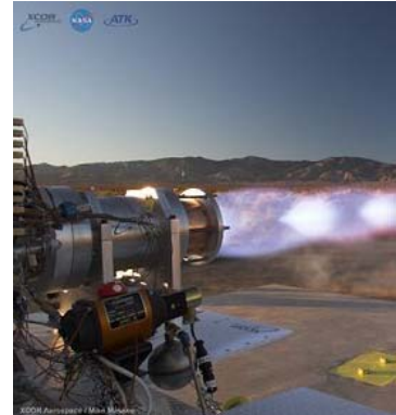
Test firing of a 7,500 pound-thrust LOX/methane engine. Image credit: Mike Maseel/ XCOR Aerospace
