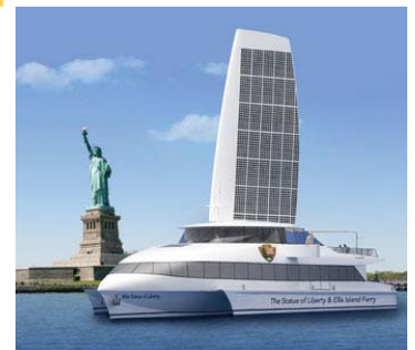
Circle Line's state-of-the-art solar and wind powered hybrid electric ferry named Miss Statue of Liberty. Photo credit: Solar Sailor
