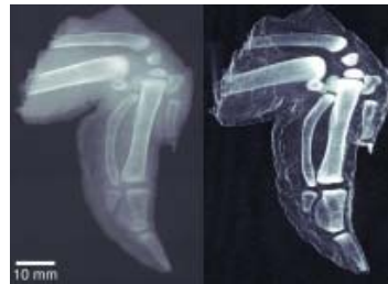
Traditional x-ray image of chicken wing on left; more detailed darkfield image on right. (Image Source: EPFL)
