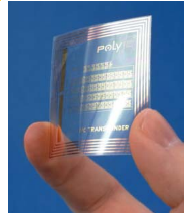
Model of a polymer flexible RFID tag. (Image Credit: PolyIC press picture)
