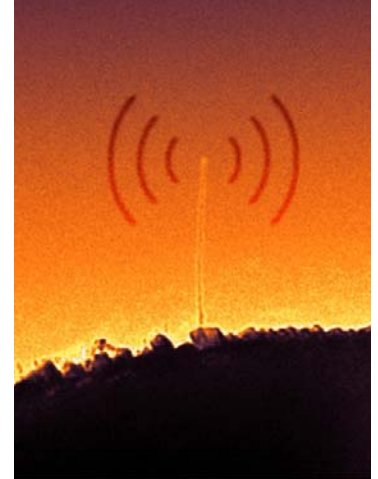
This image, taken by a transmission electron microscope, shows a single carbon nanotube protruding from an electrode. The waves shown were added for visual effect.
